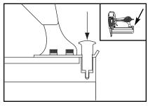
Figure 1. Releasing magazine latch.
